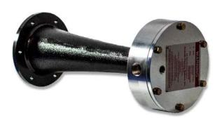
ACS acoustic cleaners use compressed air to flex a titanium diaphragm to produce pressure pulses that are amplified by the bell. The resulting low frequency/high energy sound waves that are emitted resonates/dislodges particulate deposits. The displaced particulate deposits are then removed by gravity and/or gas flow.
